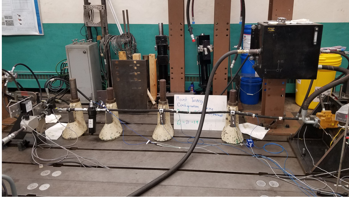
Figure 3.1: 2.13 m Hose Hydraulic Test Circuit for Mount Energy Loss Tests
